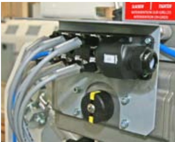
Splitter box for a quick connection to the supervision
