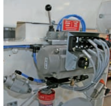
Rotative cylinder for feeding flap orientation
