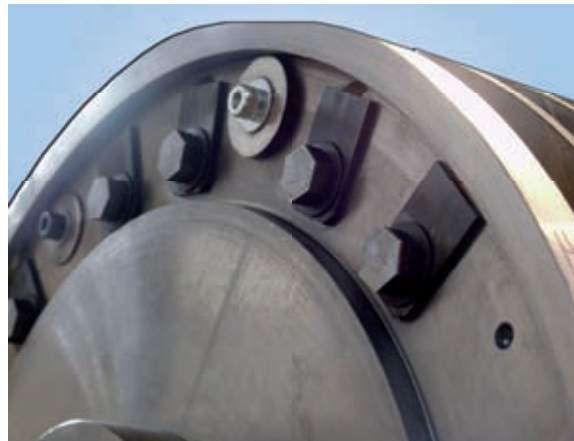
Balancing weights screwed on a hammermill rotor
