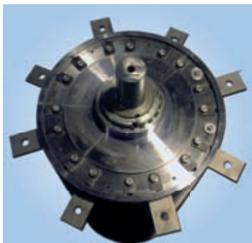
Rotor equipped with 8 rows of hammers
