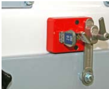
Interlocking system by key transfer
