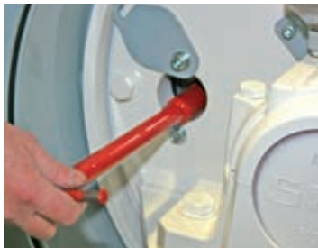
Fast exchange of hammers axles with supplied specific tools
