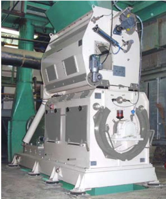
Hammermill with pneumatic conveying The most widely used for fine grinding lines (0.8 mm or 20 mesh screens)
