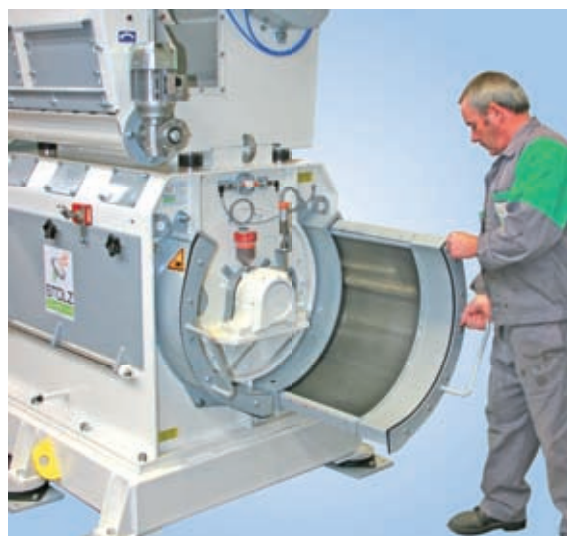
Manual change of operating screens protected by guard
