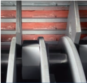
Grooved armor plate inside the grinding chamber
