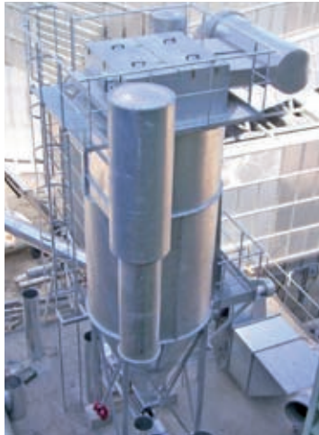
Galvanized cyclofilter with sleeves
