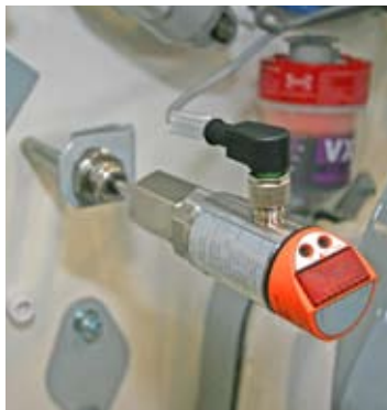
Temperature gauge on grinding chamber
