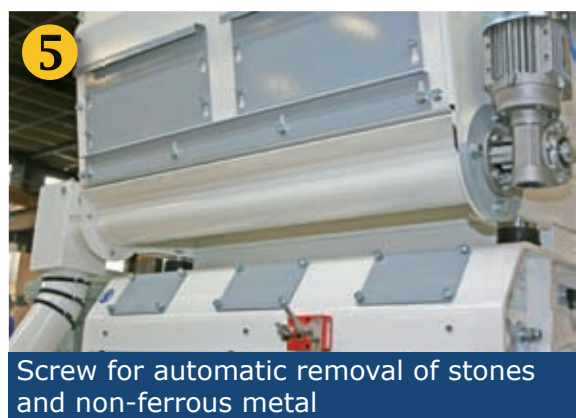
Magnetic separator with automatic cleaning
