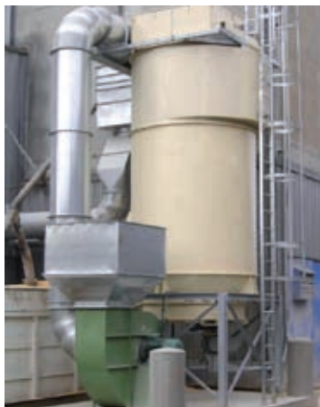
Cyclofilter with pneumatic conveying
