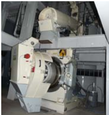
Super conditioner in pellet mill preparation
