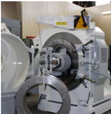
Built-in winch for die handling
