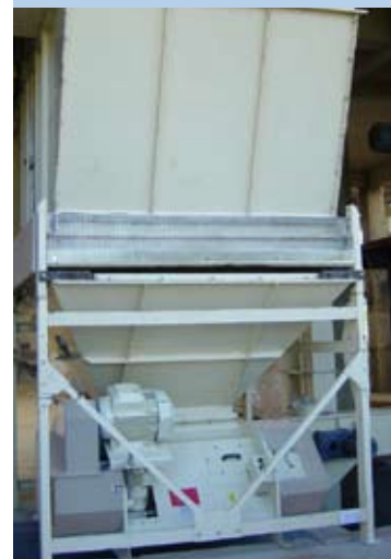
Crumbler beneath cooler
