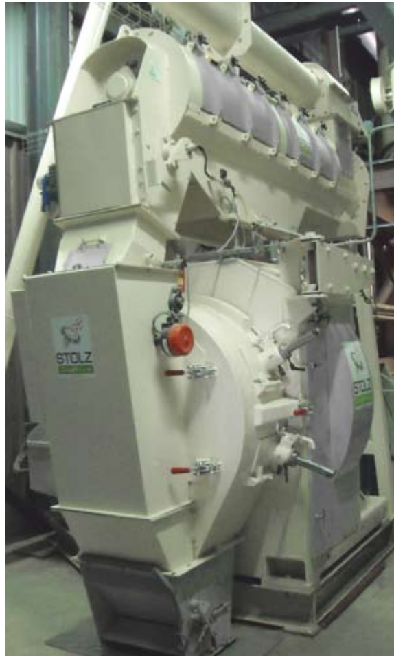
Long residence time horizontal conditioner on pellet mill
