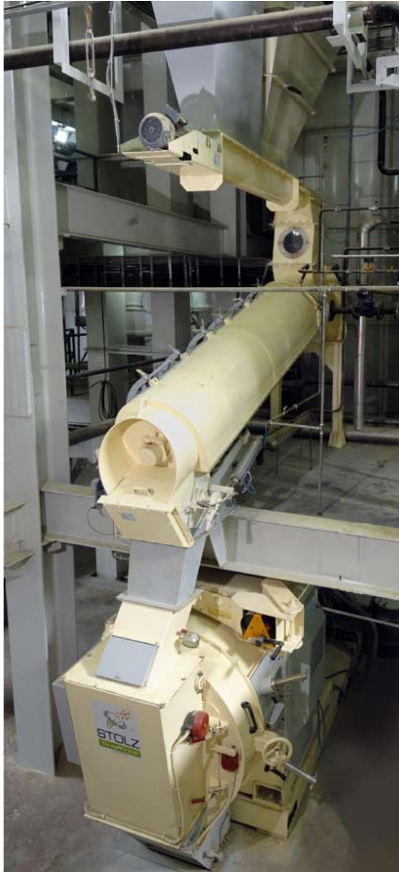
Super conditioner upstream a pellet mill
