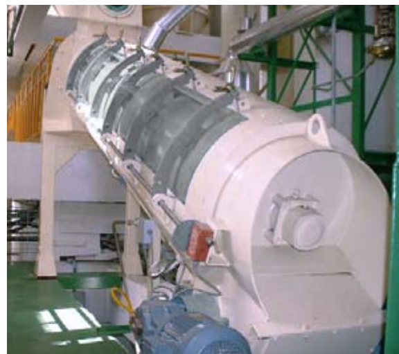
Super conditioner in pellet mill preparation
