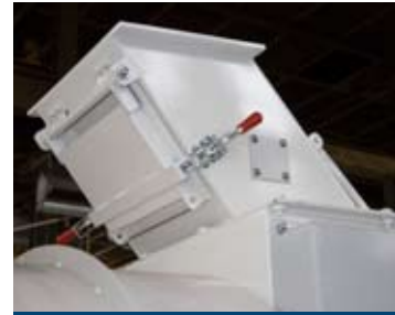
Magnet on feed chute
