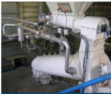
Super conditioner with steam injection
